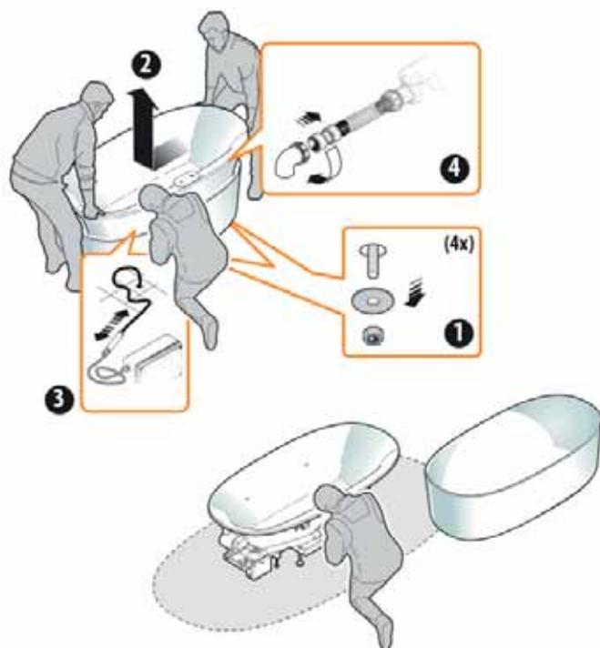
■ Tub fixing system with brackets (S)
